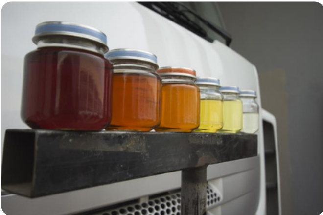
Above: Various stages of regenerated transformer oil
